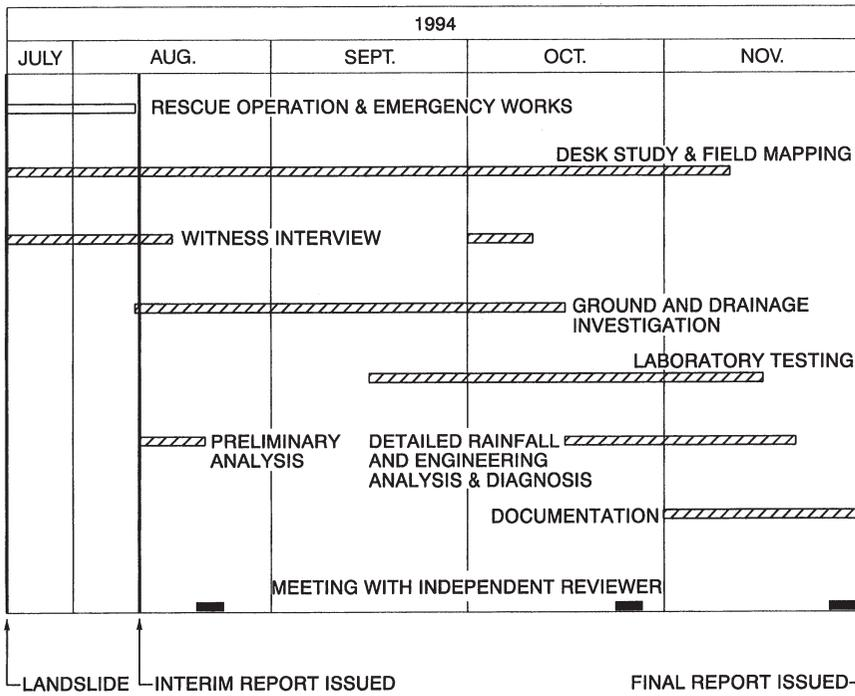
Figure 2. Programme of the Kwun Lung Lau landslide investigation
